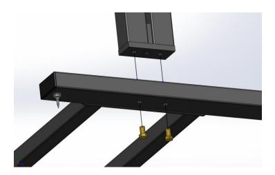
4. Fasten a Motor Cradle to the top of each riser by using the 7/16-14 x 1 Flat Head Cap Screws. Ensure the holes specified in the drawing are oriented toward the back of the stand to ensure the motor can be mounted properly.
