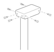
Use all 6 threaded mounting holes M6 for screws. Thrust moment is 7.5Nm
