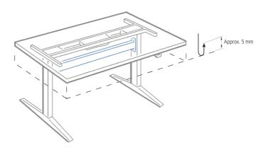
The CBD5 and CBD6 can control DL5 and DL6 in 2 parallel while the CBD4 can control DL5 and DL6 in 2, 3, and 4 parallel so that the desk is always kept horizontal.
