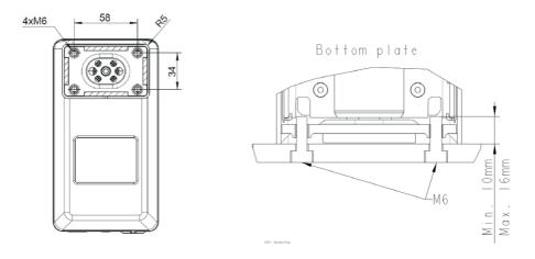
The 4 holes in the bottom of the column are placed from each other 58/34 mm respectively.
