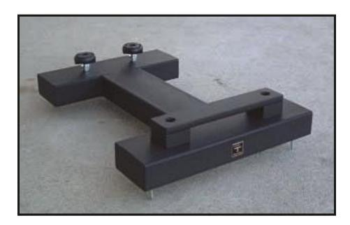
Sound Anchor 801 / 802 Nautilus Stands do not fasten to the speakers. The speaker simply sits on top of the stand with four specially chosen points of contact. The two holes in the front cross bar locate and support the front of the speaker on the stand. The two industrial grade adjustable leveling pads support the rear of the speaker. These pads can be adjusted to level or tilt the speaker backward or forward.
